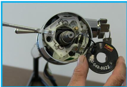
3. Then, slide the Canceling Cam over the column shaft and canceling cam spring. *For proper operation of the canceling cam, align the canceling cam stem between the 10 and 11 o'clock position. (figure A)*
