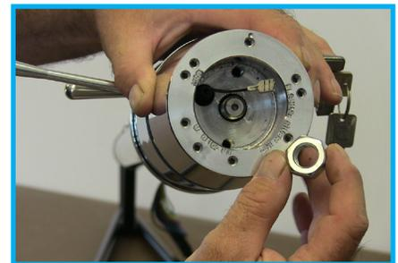
5. When installing your steering wheel adapter, tighten the retaining nut to 50 ft lbs.
