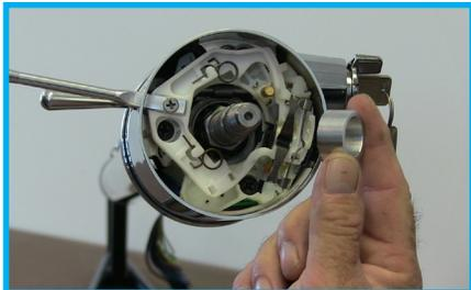
1. Install the large 5/8" aluminum spacer over the column shaft.
