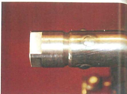
*I started by doing the rosette welds first, then going back and filling the V where the machined end met the beveled end of the extension tube.*
