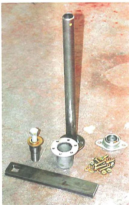
*The conversion consists of an output shaft adapter that's splined to match either a reversed OE Corvair box or a Flaming River reversed box, an extension shaft that bolts to the adapter, a machined end piece for the shaft, and a straight cut Pitman arm. They also suggest the use of a shaft support (which they can supply as well) which will reduce the torsional twist on the steering box mounting bracket and output shaft.*
