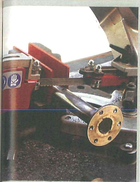
Once marked I used my band saw to cut it to length and then drilled the rosette holes in the end. Also keep in mind that you'll want to bevel the edge of the shaft for good weld penetration when attaching the machined end to the tube.
