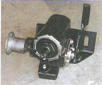
With the mounting bracket complete enough to locate the box, the next step was to mount the output shaft adapter to the box using the nut and lock washer supplied with the steering box. The mounting bracket will be reinforced for added strength after the balance of the install is complete.
