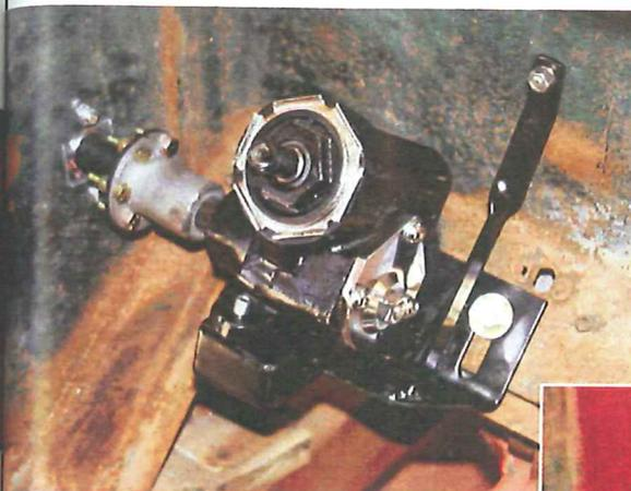
*Next, I attached the Pitman arm to the shaft using the Grade-8 bolt, flat, and lock washer supplied in the conversion kit. Gas Alley suggests the use of thread locking compound on the bolt threads as well as drilling its hex head for safety wire too. I will do both before the truck hits the road!*
