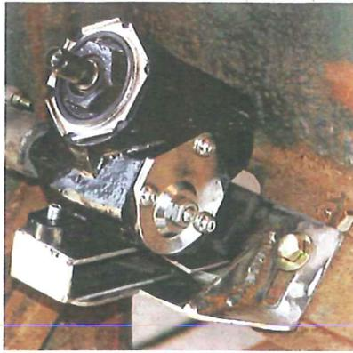
After two or three false starts I finally ended up sewing together a mounting bracket that located the box both in the correct position and solidly. Like I said, though the conversion components can be used to install a reversed Corvair box for cowl-steer in any situation, mounting the actual box will vary from vehicle to vehicle.
