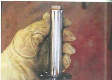
*Once the welding was completed I carefully ground the welds smooth—taking my time so as not to damage the extension tube.*
