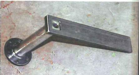
*Before proceeding I took a few minutes to test fit the Pitman arm and then to prime and paint it and the shaft before reattaching it to the output shaft adapter.*
