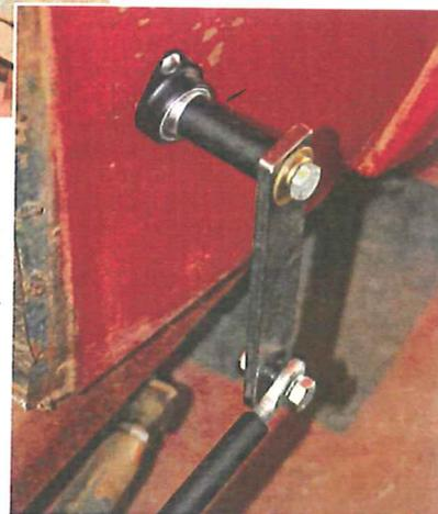
*Finally I fashioned a drag link out of a section of 3/4-inch-od DOM tubing and a pair of rod ends (those with a sharp eye may notice I hadn't added the jamb nuts) to finish off the install.*
