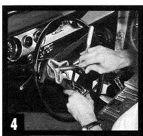
There are threaded holes in the steering wheel that allow you to attach the puller. Once the tool is in place, use a wrench or ratchet to screw the threaded center rod down to press on the column end, and the wheel will slide off.
