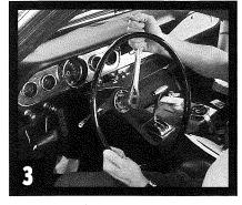
Start the steering R and R by removing the steering wheel. Push the horn button all the way to the seat, then rotate counterclockwise to remove. Next, remove the retaining nut that holds the wheel onto the column. It's tight, so hold firmly onto the steering wheel.
