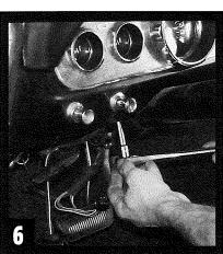
Remove the column support bracket from threaded studs, one on each side.
