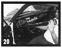
When reinstalling the column tube, be patient with the column support bracket. The nuts up top are not tack welded into place, but rather are captive in a small housing. This is so they can be moved around to provide adjustment, but it can make it a little difficult getting your threads started.
