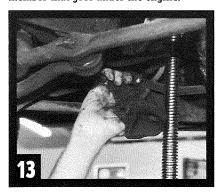
Next, the support casting that goes between the motor mount and framerail had to be removed.
