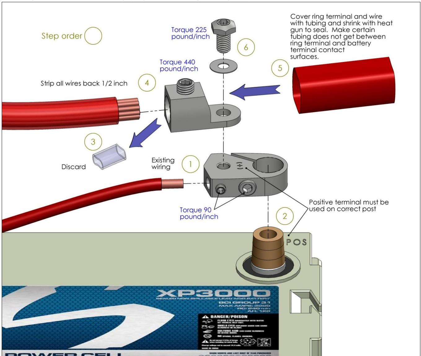
It is recommended a small amount of blue LOCTITE® be used on each ring terminal above screw. Do not get LOCTITE® on electrical connection surfaces because it is nonconductive.
