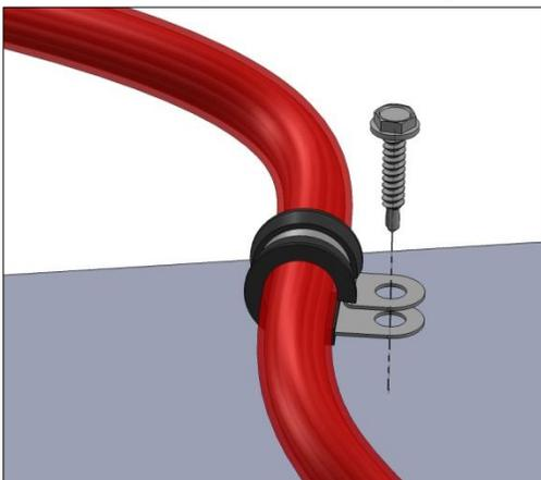
Use provided self drilling/tapping screws and insulated mounting clamps to secure cables to the vehicle. For thicker mounting surfaces, pre-drilling will be required.
