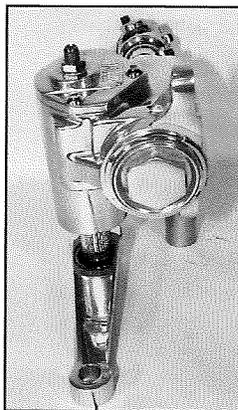
Steering boxes are available in two ratios: the original 20:1 and a quicker 16:1. To visualize the difference, here, a quick-ratio box is in the straight-ahead position.
