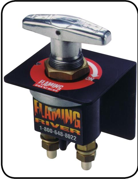
“The Big Switch” is a durable, heavy duty waterproof disconnect switch. It is designed to completely shut-off current flow from the battery of any engine-powered vehicle or electronically-powered accessory system. Rated at 250 amps at 12V and 24V for continuous service (2,500 amps for 5 seconds). “The Big Switch” is applicable to virtually any 6, 12 or 24 volt electrical system. It can be used as an emergency cut-off switch, anti-theft device, or a simple on/off switch.
