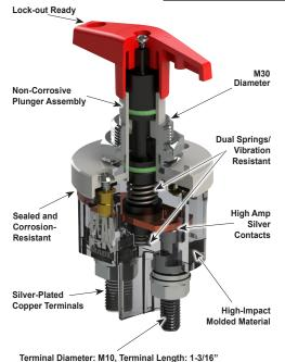
To activate switch, push handle down while turning
